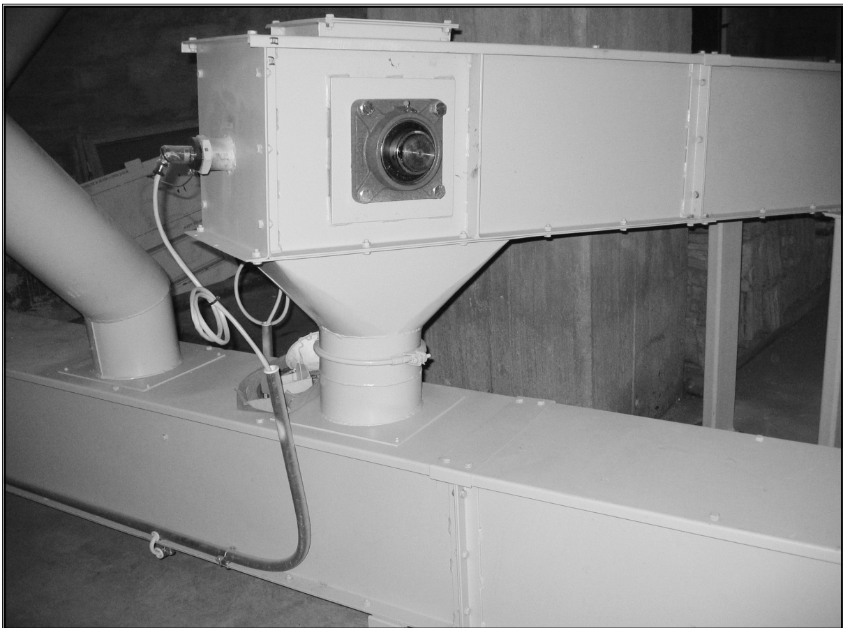
Picture 2. Jam detector in conveyor's driving end.
