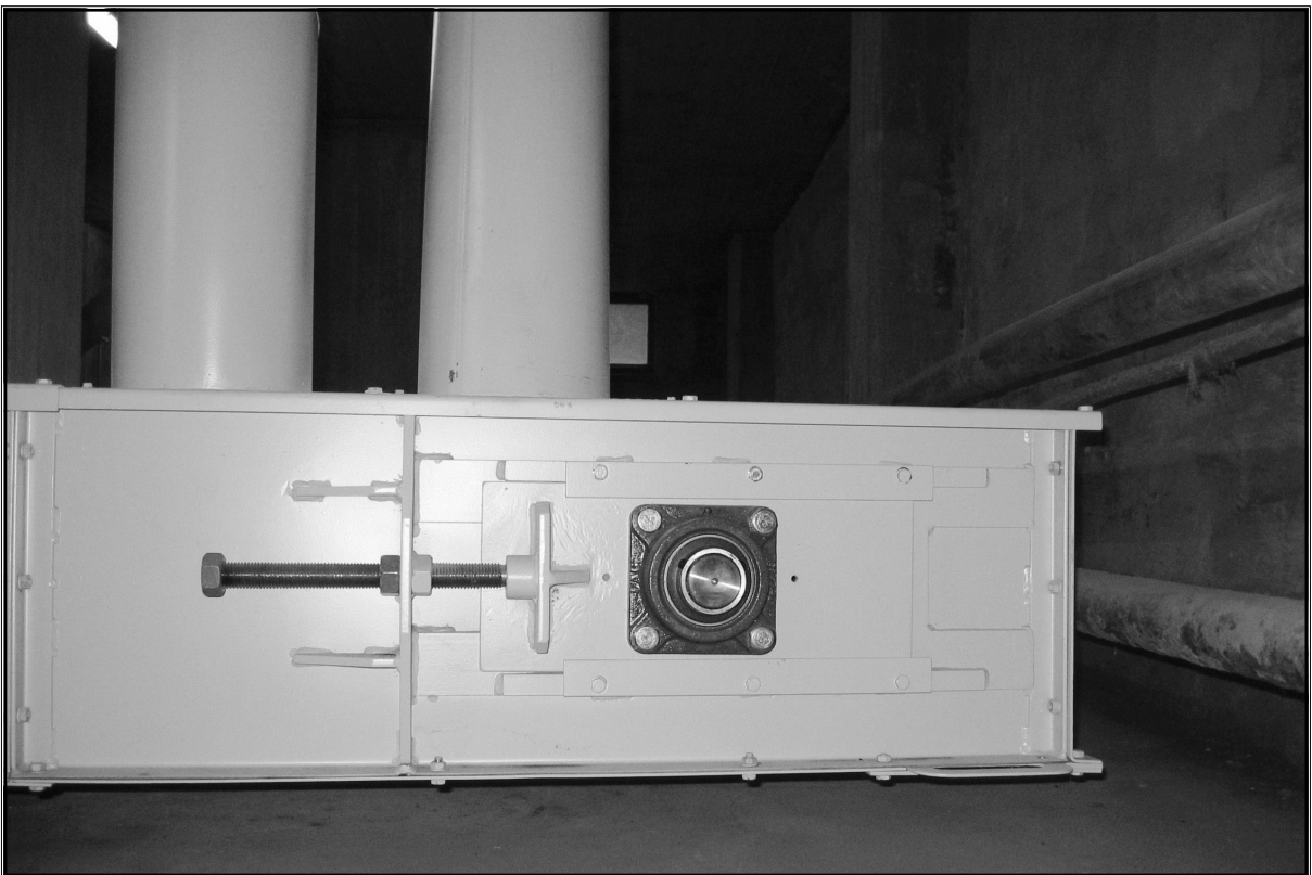
Picture 4. Folding end housing, trimming plate, trimmings screw and collar step bearing.
